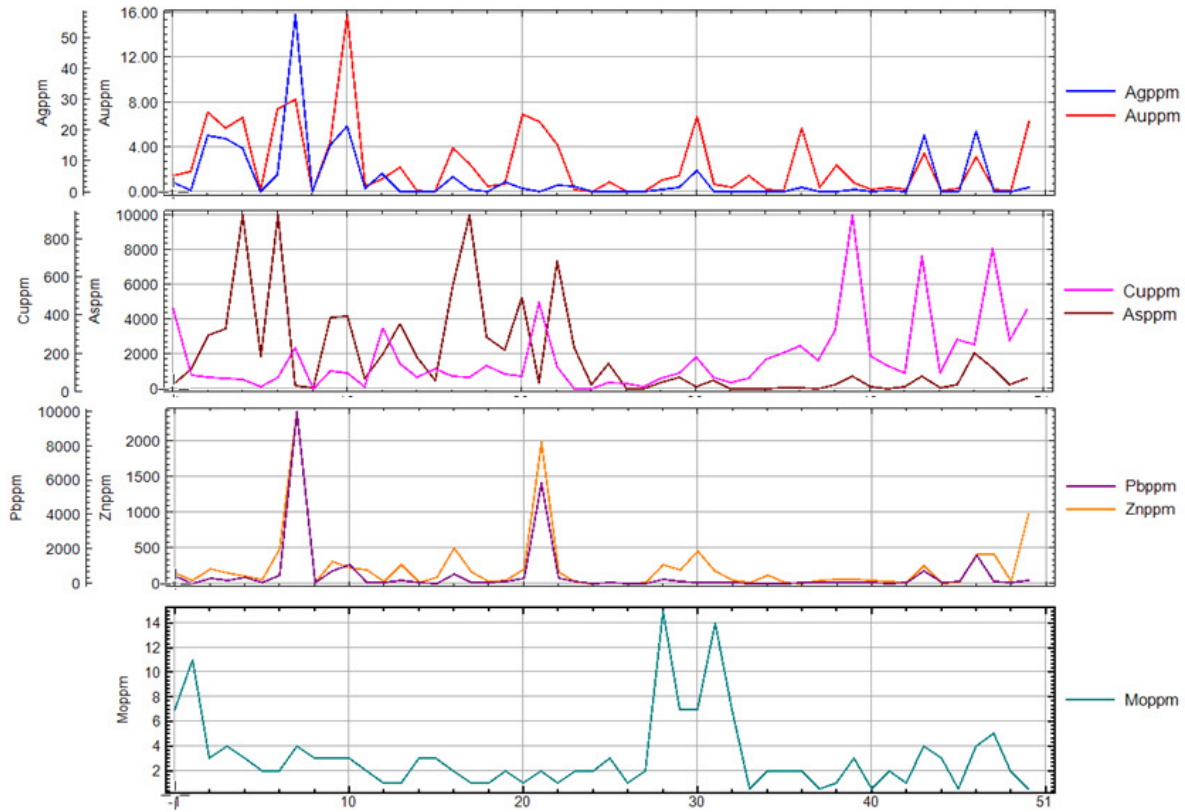
Figure 8: Au, Ag, As, Cu, Pb, Zn Profiles of 50 Vein-Rock Samples of Bolsa el Diablo (Los Incas 2009)
